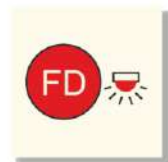
Space Protected by Automatic Fire Alarm
