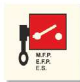
Remote Fire Pumps or Emergency Switches
